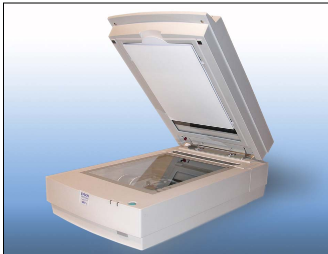
Fig. 3: An ordinary image scanner can be used as a powerful detection instrument.
